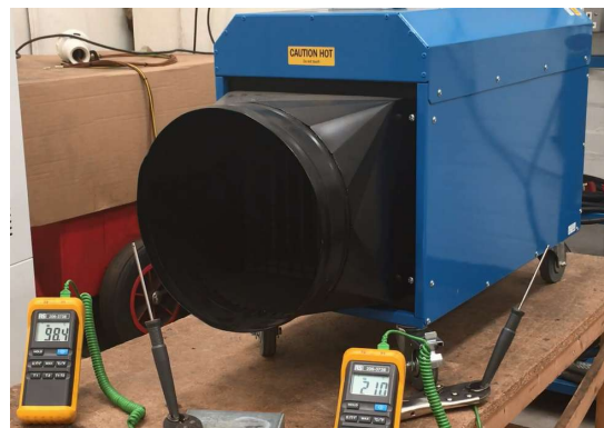
Thermostatic probes demonstrating the impressive temperature rise
